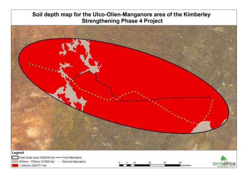
Figure 5: Soil depth map for the Ulco-Olien-Manganore area of the Kimberley Strengthening Phase 4 Project
